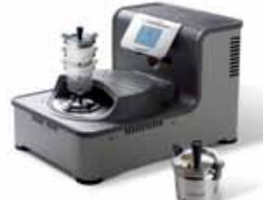
**PULVERISETTE 6 premium line** – planetarni mono mlin
